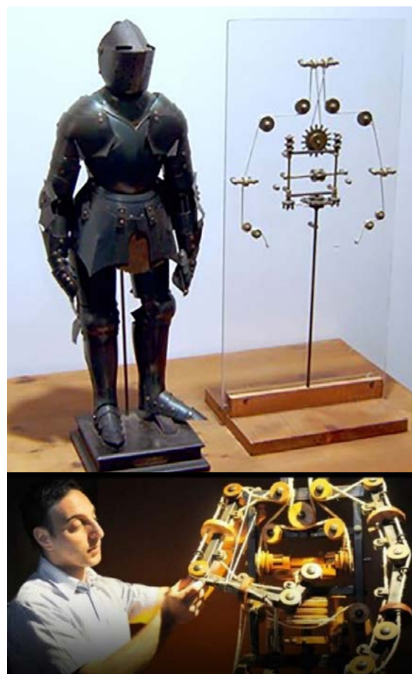
Figure 1: Leonardo da Vinci's robotic knight (1494); inset shows the fully functional model (2002) of da Vinci's sketches
